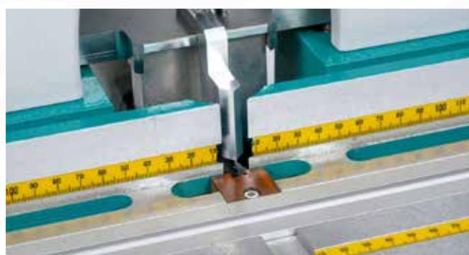
Transportable and flexible table machine, route one keyway for each swallow rate for the dovetail sizes W 0 / 1 / 2 / 3 / 4.
